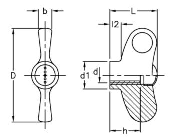
$\begin{array}{lll} b & = 10 \\ D & = 70 \\ d1 & = 20.0 \\ d & 6H = M10 \\ h & = 20 \\ L & = 36 \\ l2 & = 8.0 \end{array}$
